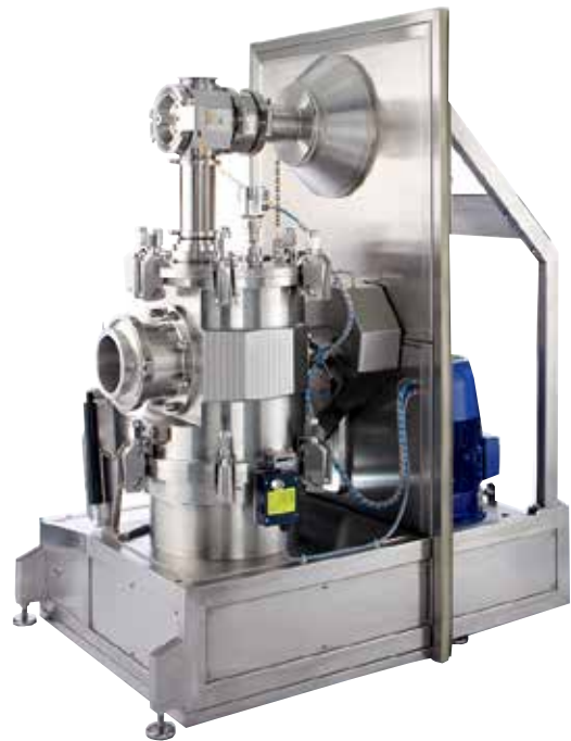
200 ZPS Maschine for Integration in Cleanroom wall
