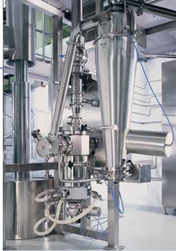
200 AFG Installation for pharma lactose
