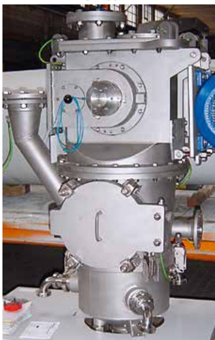
200/400 TTG WITH TURBO TWIN CLASSIFIER HEAD
